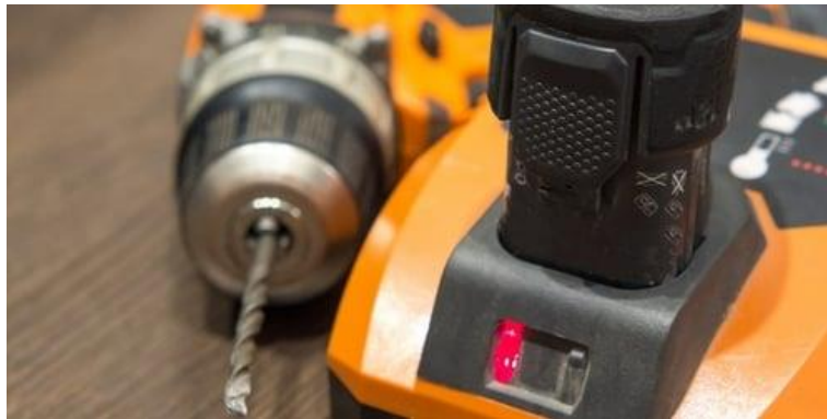
Figure 1: Lithium-ion battery for power drill on charge
